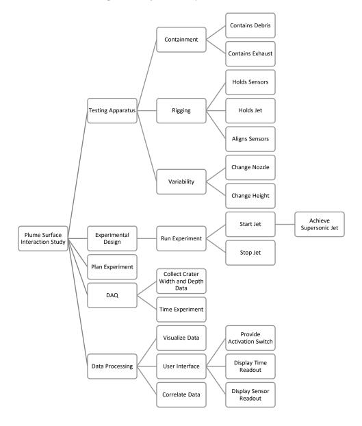
The major functions and features of the study are the testing apparatus, the experimental design, and the data processing. These were determined by considering which aspects of the test would be necessary to ensure substantive results that upheld both the team's standard and the requests of the project sponsor. The subfunctions are a further breakdown of what is needed for the major functions to succeed. For the testing apparatus to perform, it must be able to maintain
